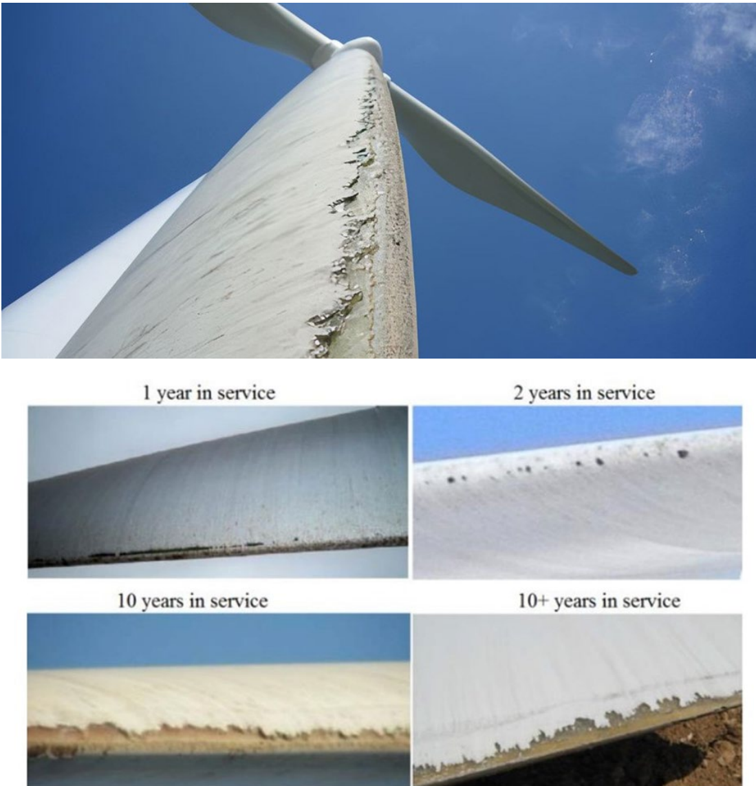
Figure 6. Examples of leading edge erosion in the field across a range of years in service. Source: [25]
